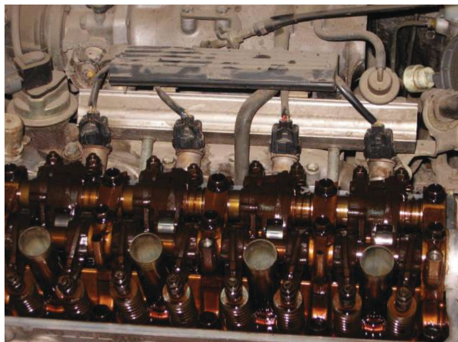
Figure 8 | Oxidation residue. (Figure courtesy of Honda.)
